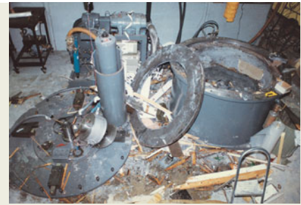
Figure 10-15 Some of the destruction caused by the explosion of a rapidly rotating steel disk.
